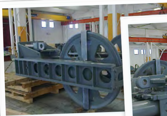
Sheaves used to move vessels and gates
