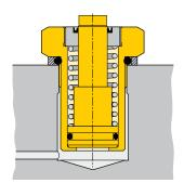
Threaded cylinders are used here to position engine manifolds for drilling, tapping and mill finish.
