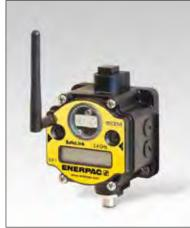
SafeLink RECEIVE units can supply the outputs by using the standard Modbus RTU RS-485 protocol. This output uses the 5 pin connector on the RECEIVE unit. If Ethernet protocol is preferred, an ETHERNET BRIDGE is available to convert the Modbus RTU R-485 to ETHERNET IP or Modbus TCP/IP.
