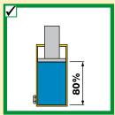
Do not operate cylinders beyond limits of rated stroke or pressure. Use only 80% of usable stroke.
