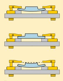
**Figure 10a**Deformation caused by conventional clamping.
