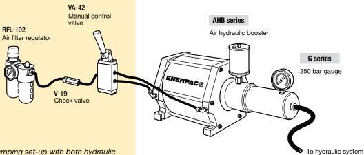
In an automated clamping set-up with both hydraulic and pneumatic components, AHB series boosters are used as a power source for the hydraulic system.
