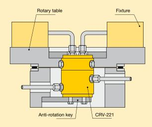
In this application eight CRV-222 rotary couplers are installed to power the individual presses of an eight station rotary press table.
