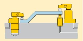
Lower flange work supports, placed close to the machining area to minimize deflection of the workpiece.
