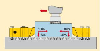
The pull down clamps can be permanently mounted using the supplied mounting bolts. Optional T-nuts can be used for adapting to varying workpiece sizes.
