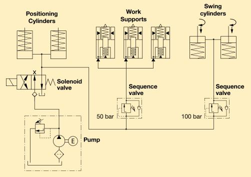
For overhanging areas of the workpiece which have to be supported, the recommended sequence should be as follows (Figure 5):
