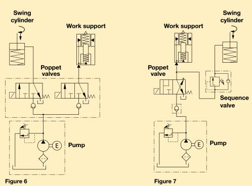
The hydraulic sequence can be controlled either by independently controlled hydraulic circuits (Figure 6) or by sequence valves (Figure 7).
