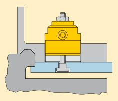
■ When pressure is released, the Enerpac MRS cylinders clamp the workpiece by pushing it against the frame that is attached to the fixture
