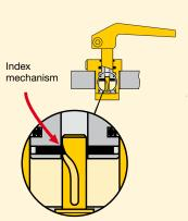
When designing custom clamp arms, the flow rates must be further reduced. This rating should be in proportion to the mass and the center of gravity of the clamp arm.
