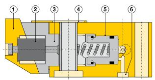
The moveable jaw ① and the flexible connection design ② allows lateral movement and eliminate any bending moment. Roller finished cylinder bore ③ improves seal life. The removable guard ④ prevents the entry of chips and allows easy cleaning. Heat treated, centerless ground plunger ⑤ for extremely close tolerances and long life. The clamps feature both manifold mount ⑥ and plumbed oil connection.
