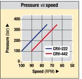
NOTES: Maximum oil flow: 9 l/min. Oil loss CRV-222 = 30 cm<sup>3</sup>/hour. Oil loss CRV-442 = 40 cm<sup>3</sup>/hour.
