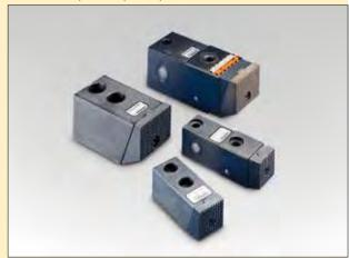
Enerpac pull down clamps are designed to allow unobstructed top face machining. Independent horizontal and vertical movement achieves high lateral and pull down forces to hold the workpiece firmly down against the machine table or fixture. The pull down forces are approximately 33% of the clamping force.
