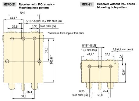
MCRC-21 with MCRA-11 Receiver with air passage and with P.O check - Mtg. hole pattern
