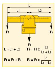
■ Two workpieces are clamped simultaneously with one doubleacting swing cylinder by using the Enerpac pivoting T-arm.
