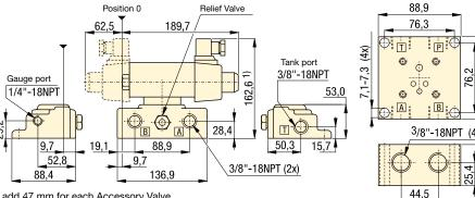
1) add 47 mm for each Accessory Valve. Note: BK-1 Bolt Kit is included with each modular valve.
