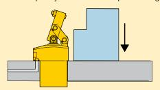
As cylinder extends, arm pivots to clamp part in place.
