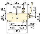
1) Manifold hole should not exceed ø 7,6 mm when port is utilized.
