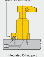
Lower flange swing clamps mounted to the face of the fixture.
