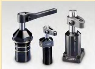
Enerpac swing clamps allow unobstructed part fixturing and placement. The plunger rod and the attached clamp arm rotate 90 degrees in either a clockwise or counter-clockwise direction, then travel down an additional distance to clamp against the fixtured part. Upon release of clamping pressure, the clamp arm rotates back 90 degrees in the opposite direction to allow for part removal and new part placement.
