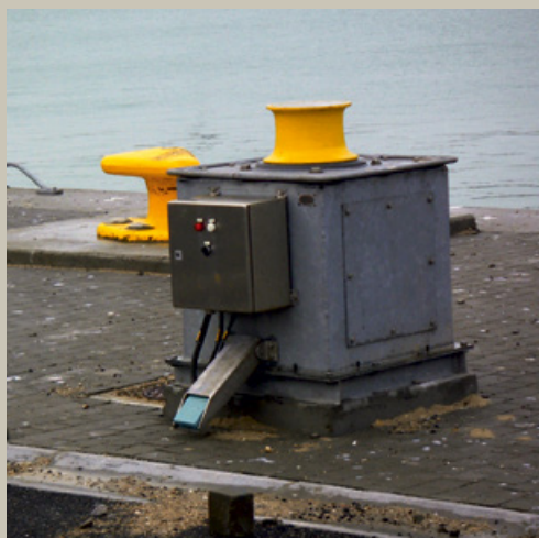
△ Capstan with foot pedal control. Capacity: 1.5 t. Speed: 25 m/min.
