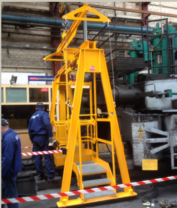
△ Gantry crane holding a nacelle used during the maintenance of a rotating laminator in which jet engine crowns are made.
