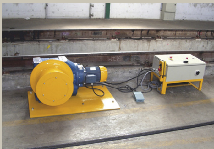
△ Horizontal capstan to pull waggons.
