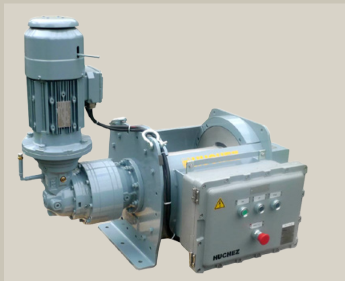
△ Lifting winch with ATEX components (electrical unit, upper and lower limit switch, motor, reduction gear).
