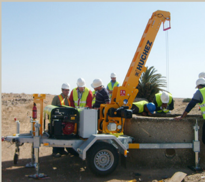
△ GMIP 140, Well Inspection Mobile Crane, used to lower engineers responsible for geological sampling into exploratory wells for mining.
